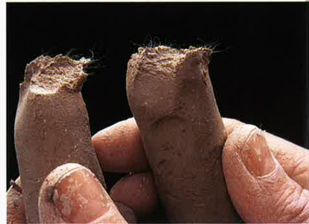
Nylon fiber in the clay body
